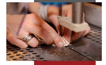
This stationary cut-off machine with fixed work table is specially designed for preparing tissue, bone and composite materials for histological evaluation and is therefore restricted exclusively for this use. A diamond-coated, high-precision cutting belt is used for cutting. The device works according to the principle of cut-thin grinding.
