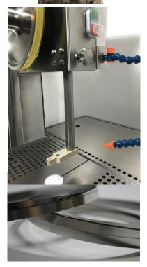
The separating strap tensioning device allows quick replacement of the bandsaw blade as well as the relaxation during longer work breaks.
